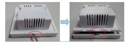
②Take the ribbon cable. Slowly open wiring seat lock, bottom line, as shown in the figure below:
